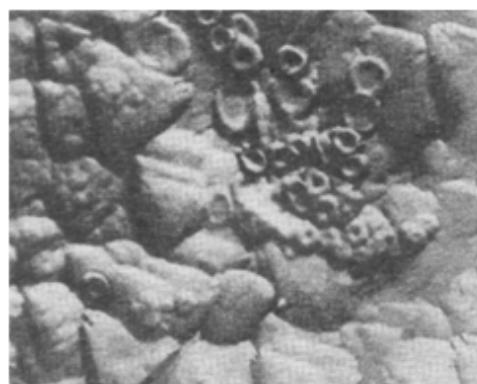
Fig.1. The dislocations and vacancy rings in  $\text{Bi}_2\text{Te}_3$  [10].
