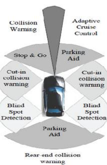
Fig. 4. Safety system using radar sensors around a vehicle.
